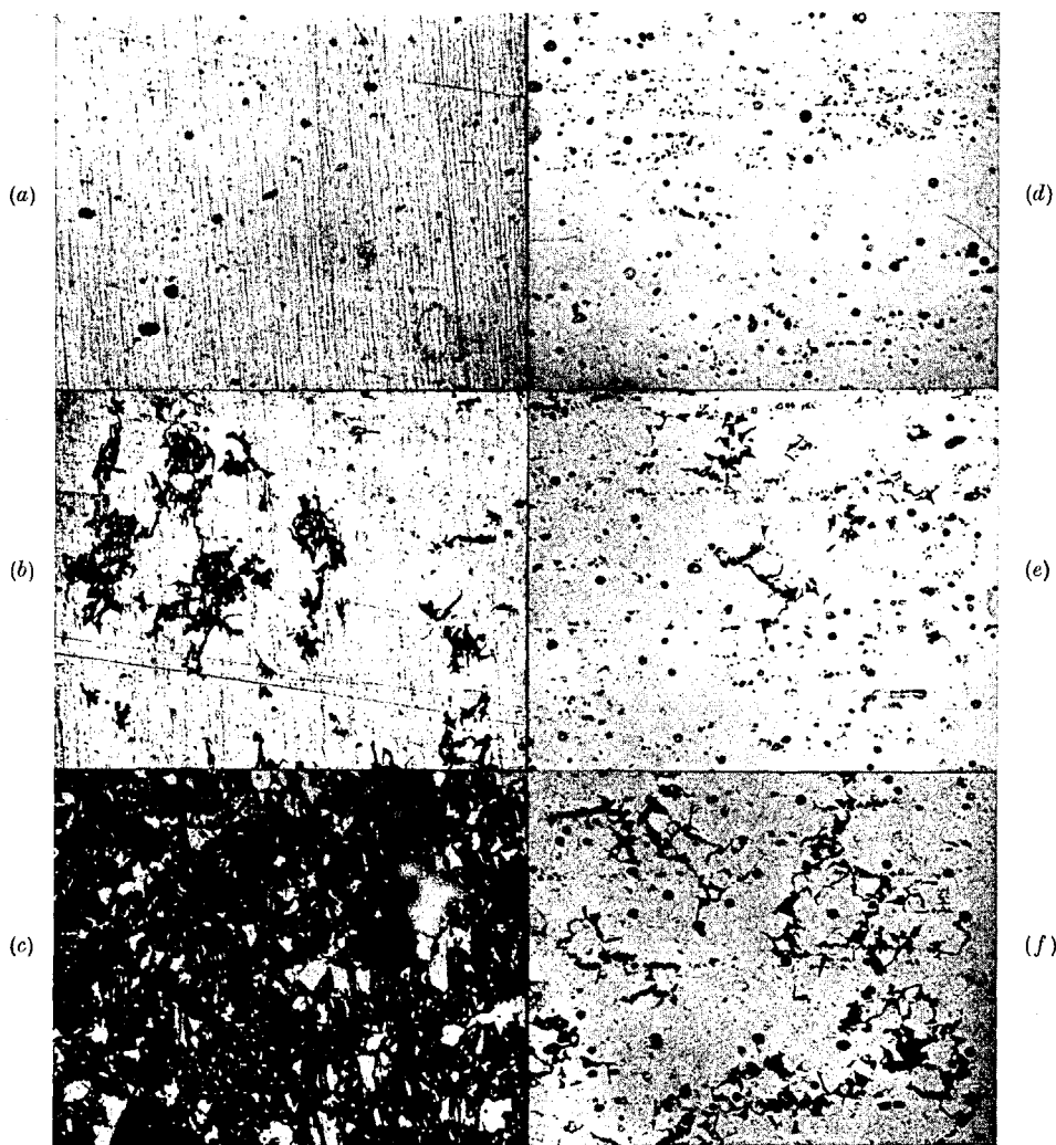
FIG. 14.—Aluminium of 99.5% Purity Rolled and then Annealed for 30 min. at 450° C. \times 63 . The surface was given a treatment in dilute NaOH solution, electrolytically polished for 10 min., then abraded mechanically on emery papers Nos. 1F, 0, and 000, under paraffin, and finally cleaned by means of benzene and alcohol. Half of the specimen was left in this condition, and the other half was electrolytically polished. The whole surface was then immersed in hydrochloric acid (13 wt.-%).
