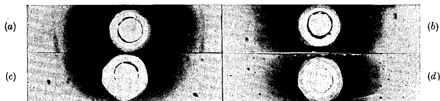
FIG. 22.—Back-Reflection Focused X-Ray Diagrams (Cu Radiation) Taken at Various Depths Below the Surface of Nimonic Alloy.
