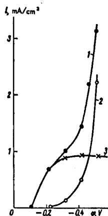
Fig. 1. Cathodic polarisation curves obtained with a gold disc electrode rotated at 2550 rev/min in NH_4SO_4 saturated with air: 1) experimental curve; 2) calculated curve for H_2 evolution; 3) calculated curve for ionisation of O_2 .
