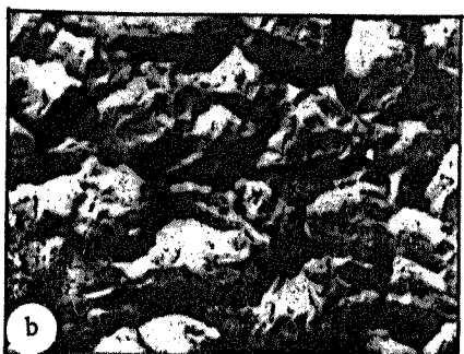
Fig. 3. Surface of a nickel deposit. Electrolyte with an admixture of (2,6 and 2,7)-disulfonaphthalic acid. 16,000 \times . a) i_{dc} = 2 \text{ amp/dm}^2 ; b) i_{dc} = 2 \text{ amp/dm}^2 ; i_{ac} = 7.5 \text{ amp/dm}^2 .
